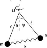
(a) Find the kinetic and potential energies and the Lagrangian for the governor.
