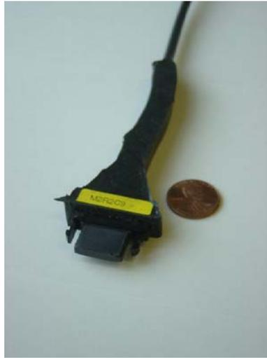
Figure 6.10: The DDK optical connector with light-tight boot made for MINERνA.
