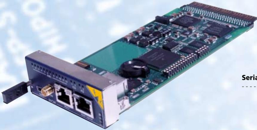
The N.A.T. MicroTCA Carrier Hub **NAT-MCH** is the central management and data switching engine for all MicroTCA systems.
