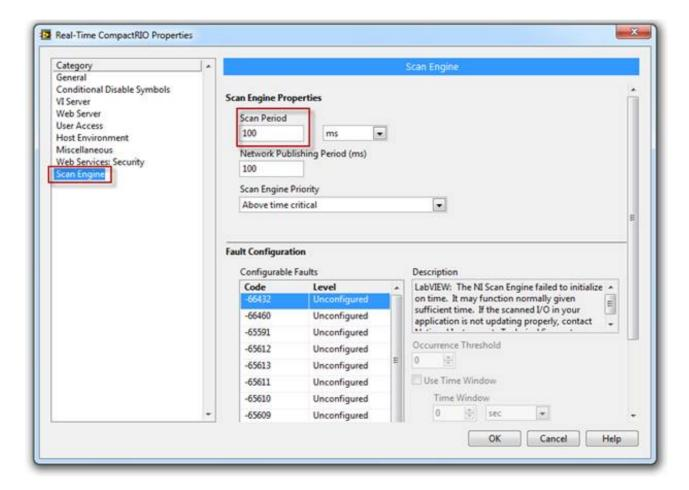
9. Now that you have configured the I/O scan rate, it is time to add the I/O reads to your application for control. When using CompactRIO Scan Mode, you can simply drag and drop the I/O variables from the LabVIEW Project to the RT block diagram. Expand the CompactRIO real-time controller, chassis, and the I/O module you would like to log. Select AIO clicking on it then drag and drop it into the timed loop on your RT.vi diagram as shown below.
