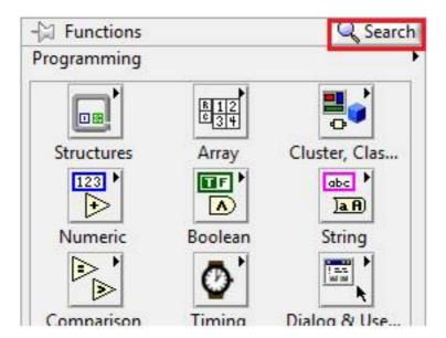
13. Search for PID and select PID.vi in the Control Design and Simulation Palette and drag it to your block diagram in the timed loop and wire the PID VI as shown in the image below.
