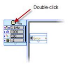
6. Select Synchronize to Scan Engine as the Loop Timing Source. Click OK. This will cause the code in the timed loop to execute once, immediately after each I/O scan, ensuring that any I/O values used in this timed loop are the most recent values.
