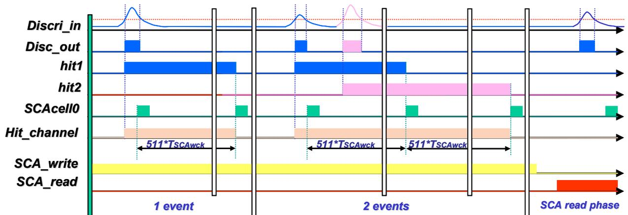
Fig 5: Hit-channel register setting.
