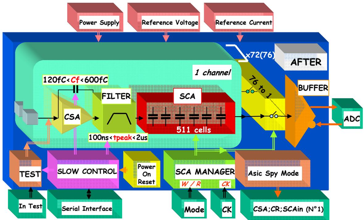
Fig 1: Block diagram of the AFTER chip.
