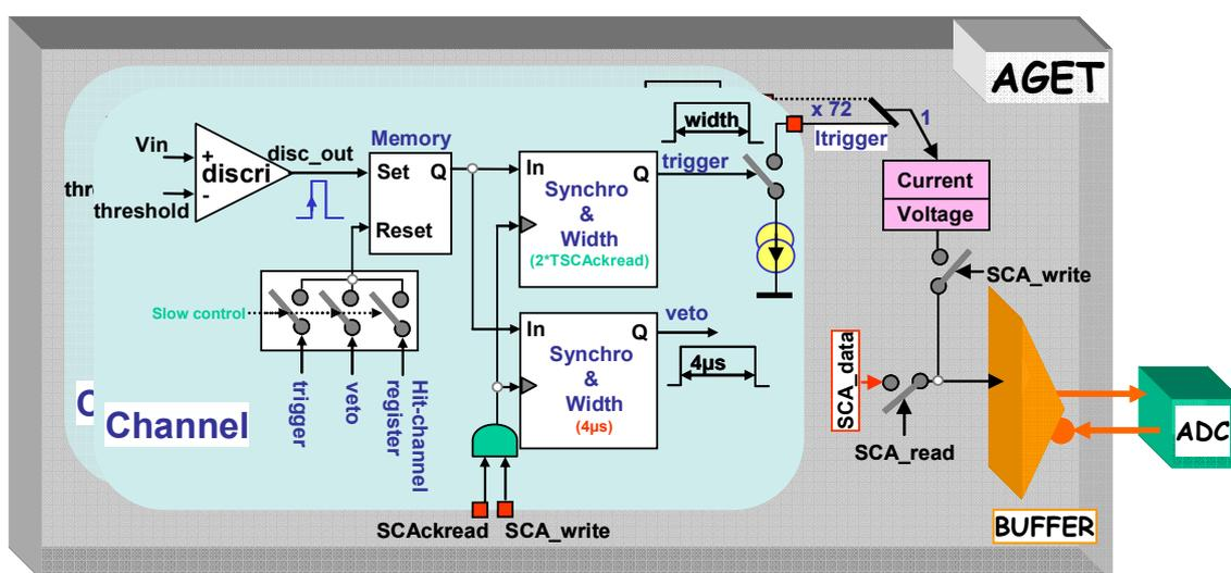
Fig 6: Principle of the trigger output.
