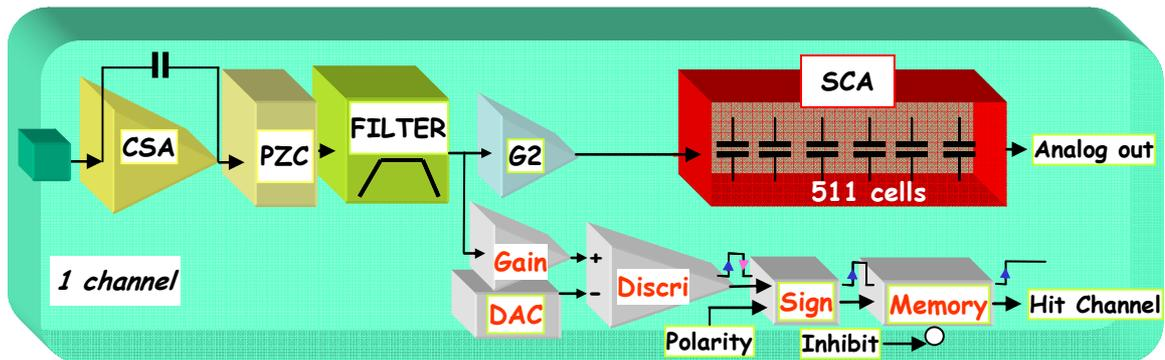
Fig 4: Block diagram of the channel.
