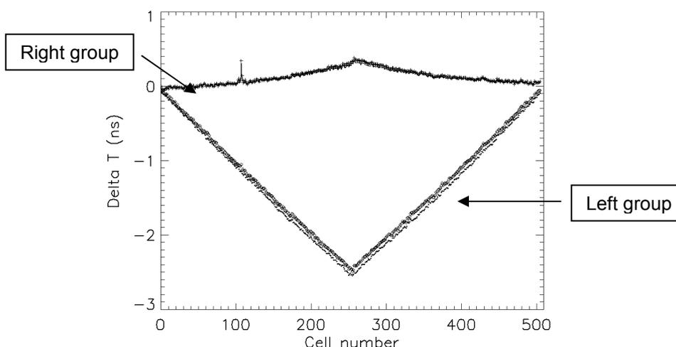
**Fig 3: Variation of the effective sampling time with the cell index in the SCA.**
