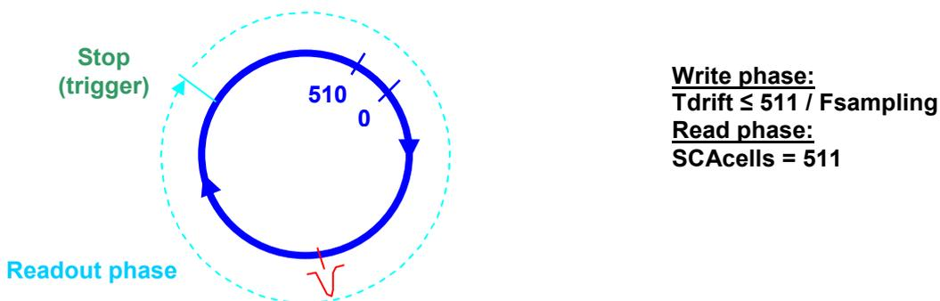
**Fig 7: 511 cells readout mode.**
