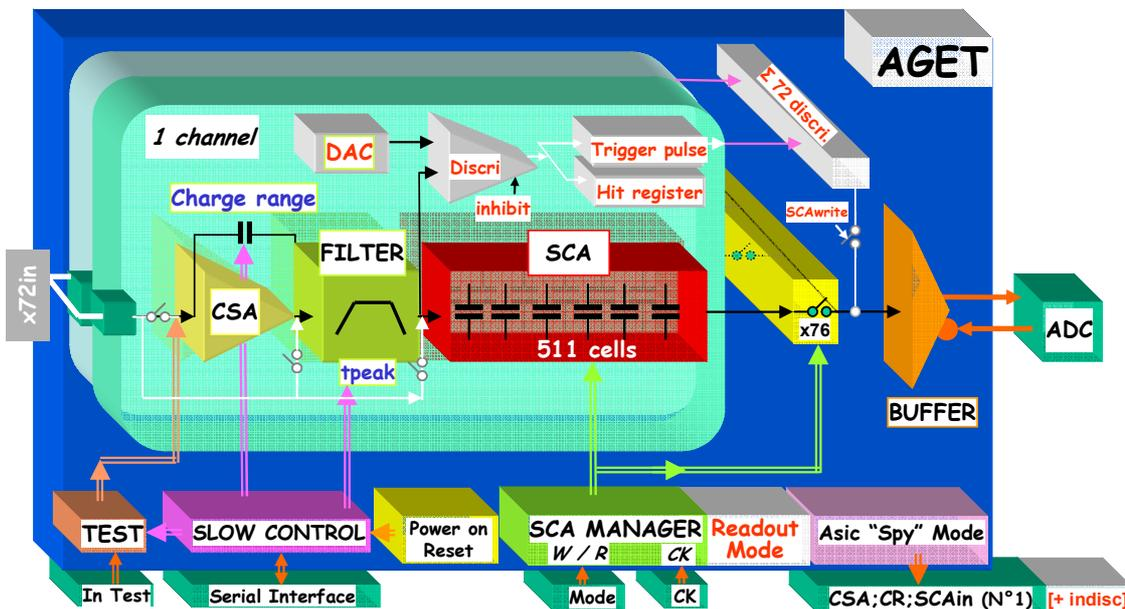
**Fig 2: Block diagram of the AGET chip.**
