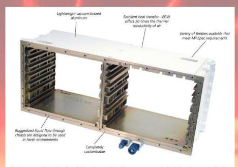
Aluminum vacuum-brazed liquid-cooled chassis are used in military, aerospace, and other high performance applications because they offer excellent heat transfer in a lightweight package. All of Lytron's liquid-cooled chassis are custom designed to match your thermal and mechanical performance, pressure drop, and dimensional requirements.
