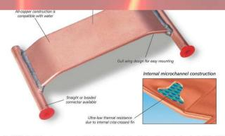
The CP25's ultra-high performance makes it ideal for high heat load applications. The standard product is 1.3" x 2.3" (33mm x 58mm), so it is an excellent solution for cooling small, high watt-density components, For large area cooling applications, the flat tube can be integrated into larger assemblies.
