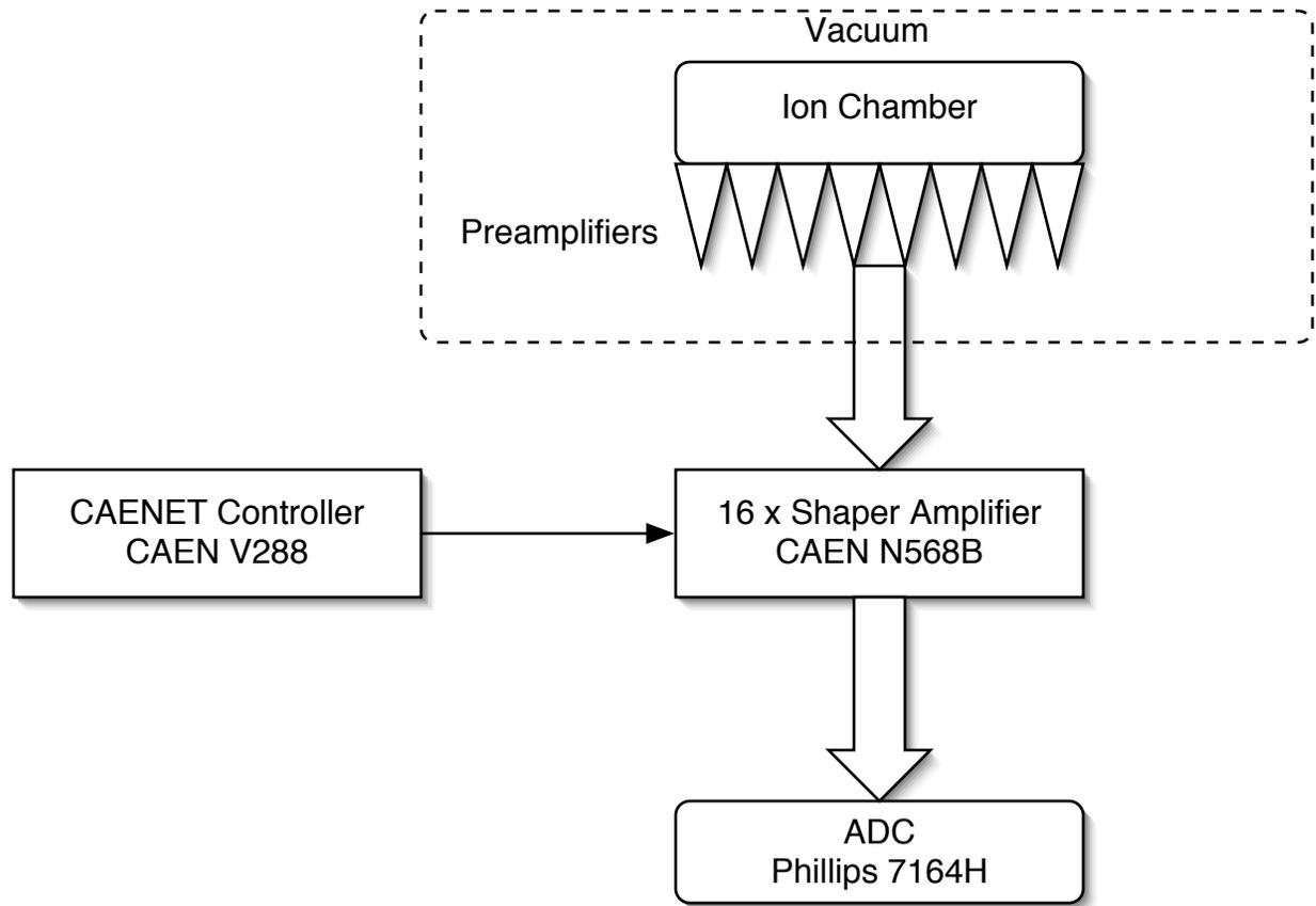
Ion Chamber Electronics Diagram
