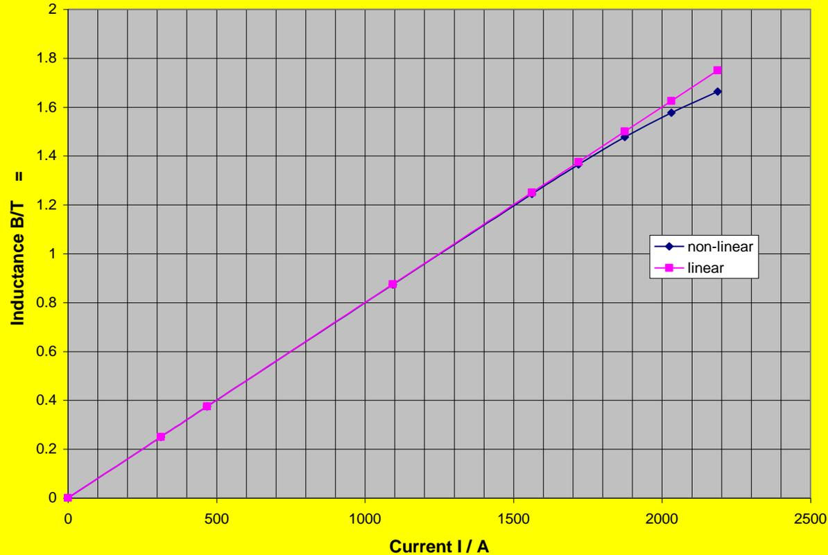
These figures show the Good-field region in the center of the magnet and the maximum field B as function of the current I in the conductor
