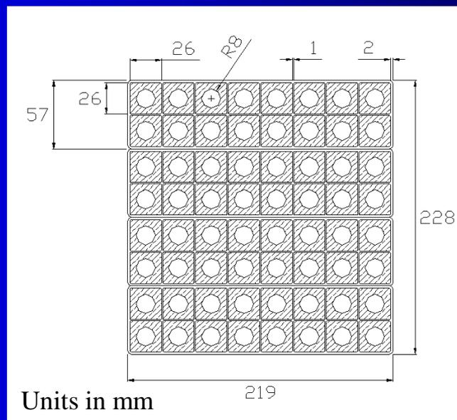
This figure shows the coil with hollow copper conductor for water cooling (4.3 A/mm<sup>2</sup>)
