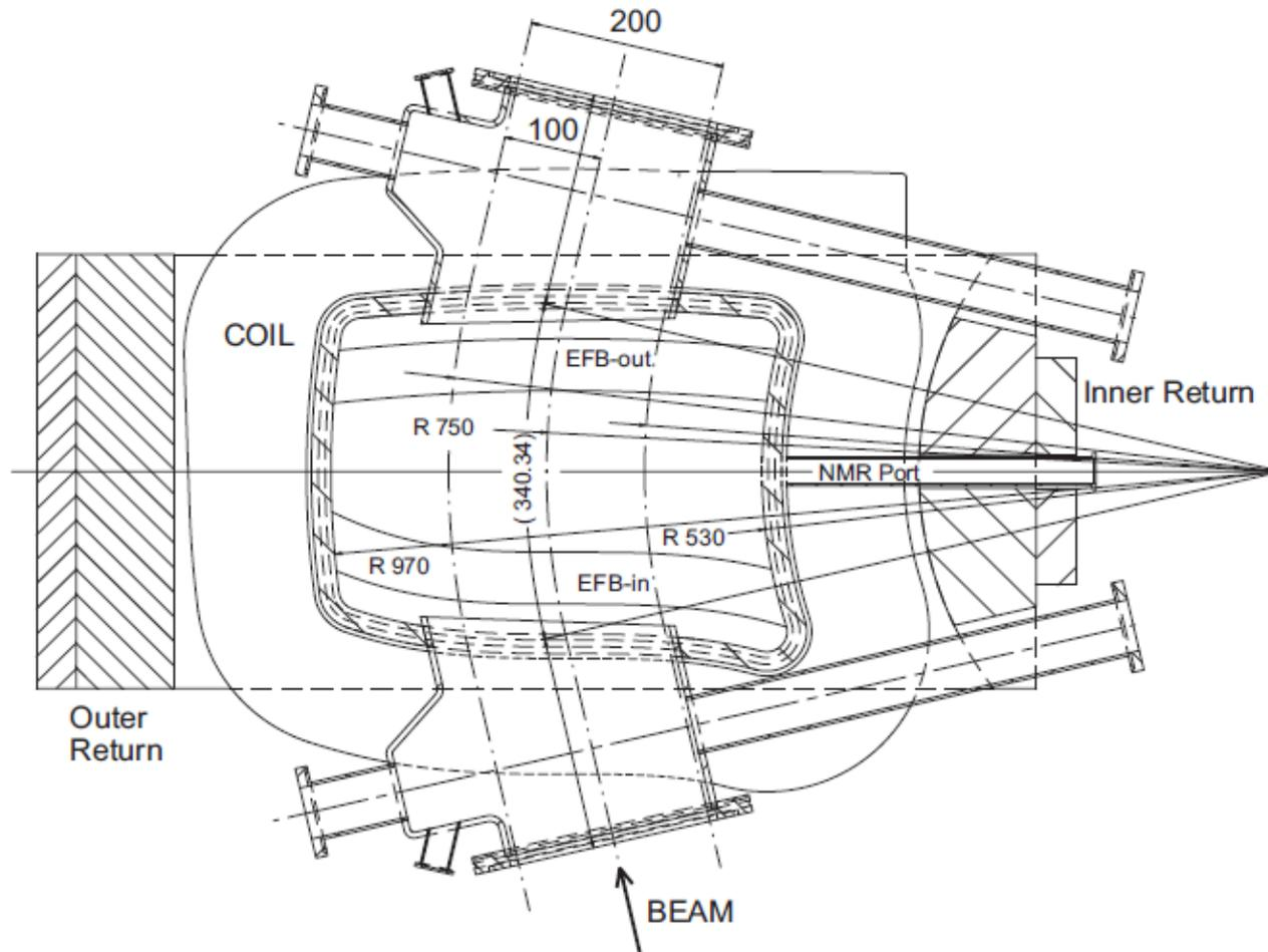
Fig. 4. View from above the midplane of dipole magnet B1 and the vacuum chamber. The physical shape of the pole piece at the entrance (EFB-in) and the exit (EFB-out) is designed to create the higher-order corrections. All dimensions are in millimeter.
