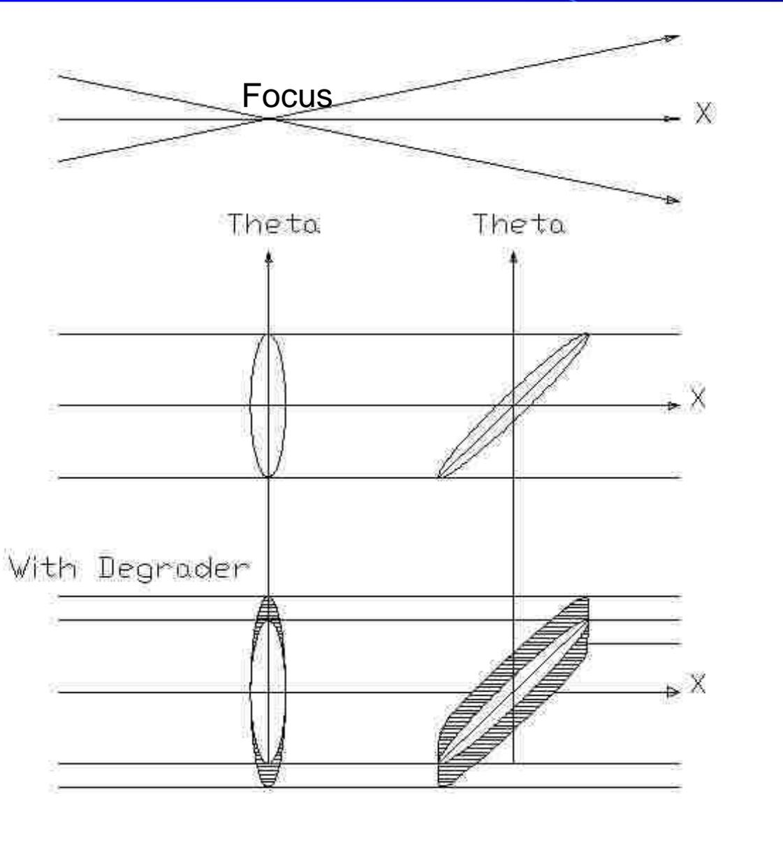
Focussing with triangular K-coil in Dipole D2
