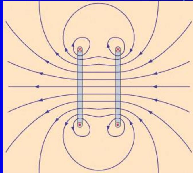
Helmholtz coil, reversed current, Quadrupole
