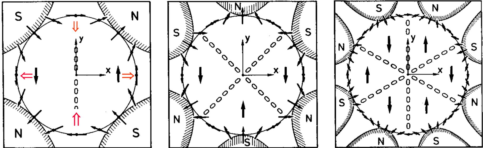
**Fig. 9.15.** Pole arrangements of magnetic quadrupoles, hexapoles, and octopoles are indicated. Also shown is a circle of radius  $r_0$  along which the magnetic flux density is constant, and its direction varies as indicated. Finally, strings of zeros indicate lines along which  $B_y$ , the y component of the magnetic flux density vanishes. These lines separate regions in which  $B_y$  is parallel or antiparallel to the y axis.
