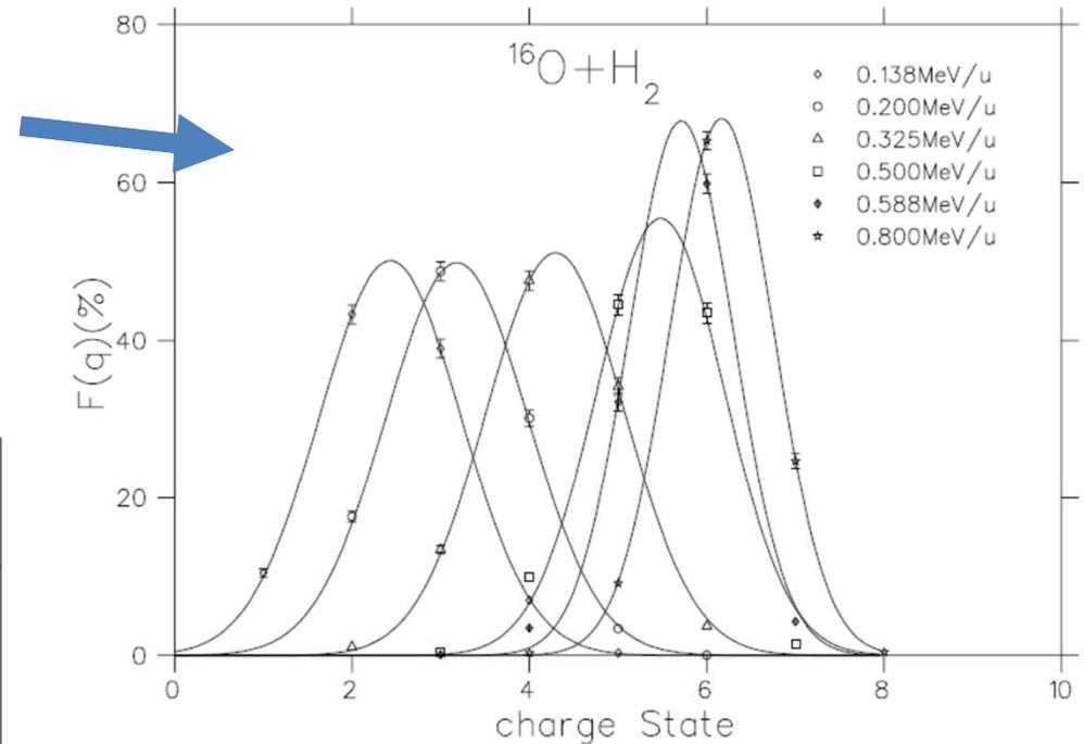
Figure 4.2: Equilibrium charge state distribution of  $^{16}\text{O}$  beam passing through hydrogen gas target, with symbols representing the experimental data and line for Gaussian distribution.
