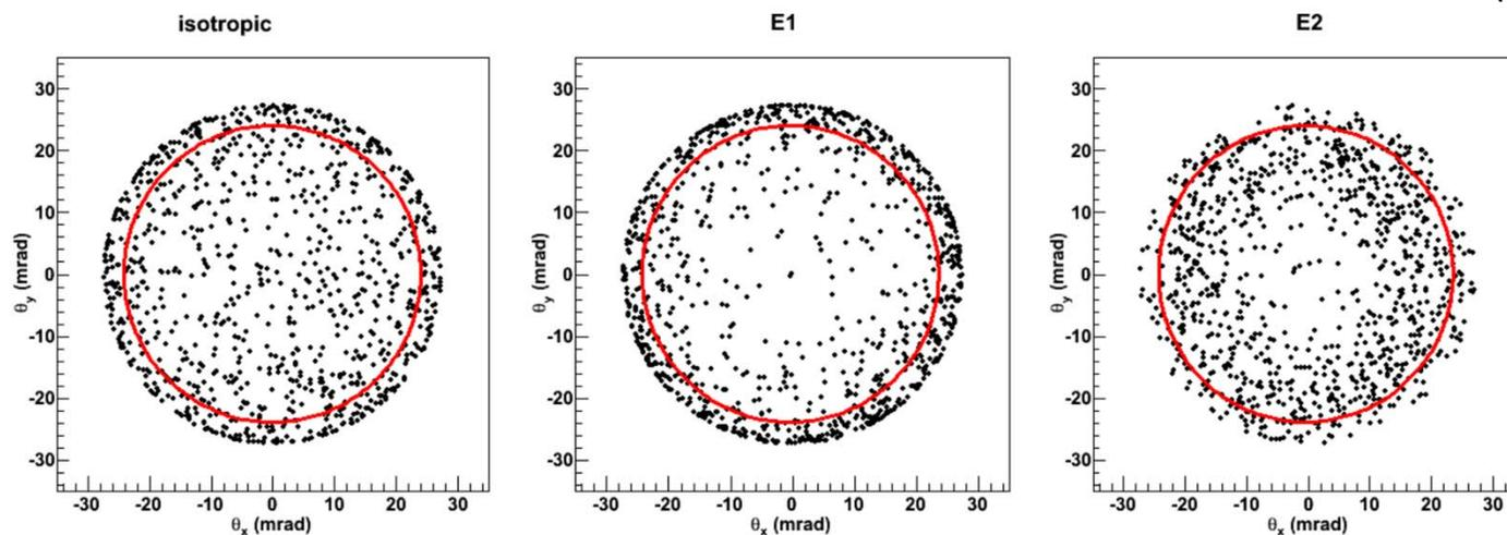
Figure 1 Distribution of recoils in the  $\theta_x$ ,  $\theta_y$  space for  $^{12}\text{C}(\alpha,\gamma)^{16}\text{O}$  ground state transition at  $E = 1.0$  MeV. For different  $\gamma$ -ray angular distributions. Left: isotropic. Center:  $\sin^2 \theta$ . Right:  $\sin^2 \theta \cos^2 \theta$ . For reference, a circle shows an angular acceptance of 24 mrad. See text for details.
