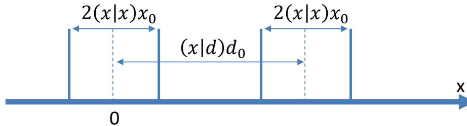
The resolving power is the inverse value of  $d_0$  that still provide a separation
